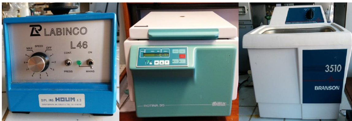
Figure 17 Picture of the three machines used for washing and isolation of the particles. From the left Labinco L 46 stirrer, Rotina 35 centrifuge and Branson 3510 sonicator
