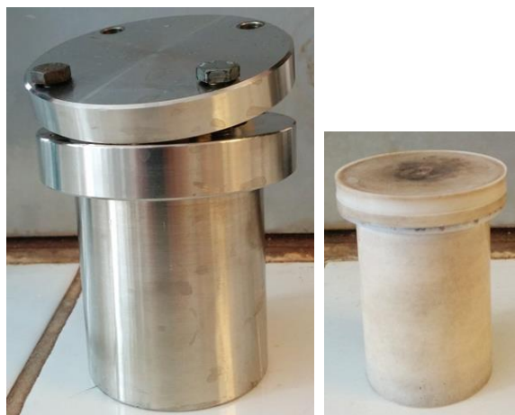
Figure 16 Picture of autoclave (left) and Teflon liner (right) used for the synthesis of the particles. The Teflon liner has an inner volume of 40 ml
