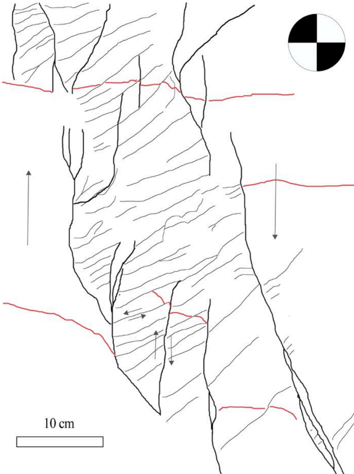
Figure 5.7: A ladder structure illustration. The illustration is drawn on the basis of a photo from Fremont bedding. The vertical, darker markings are representing thicker deformation bands. The lighter, diagonally running deformation bands are less weathering resistant. The red lines illustrate layers in the sandstone, showing direction of movement. In thin sections the diagonal deformation bands are absent of grain crushing and cementation, and therefore classified as disaggregation bands. The stress is displayed in a focal diagram in the upper right corner. The ladder structure has a normal displacement. The focal diagram shows stress areas, which may contribute to understanding the occurrence of diagonal deformation bands.
