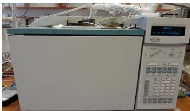
Figure 4.8: Gas chromatograph instrument, Aligent 6890 A with FID detector used to analyze the gas effelunt.
