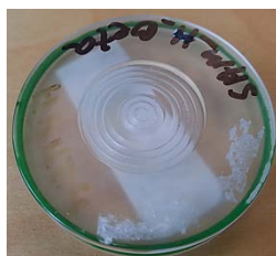
Figure 3.12: Sample holder used in powder XRD characterisation. The powder sample is placed in the center of cavity type sample holder while making the flat and smooth surface by gently pressing the powder.
