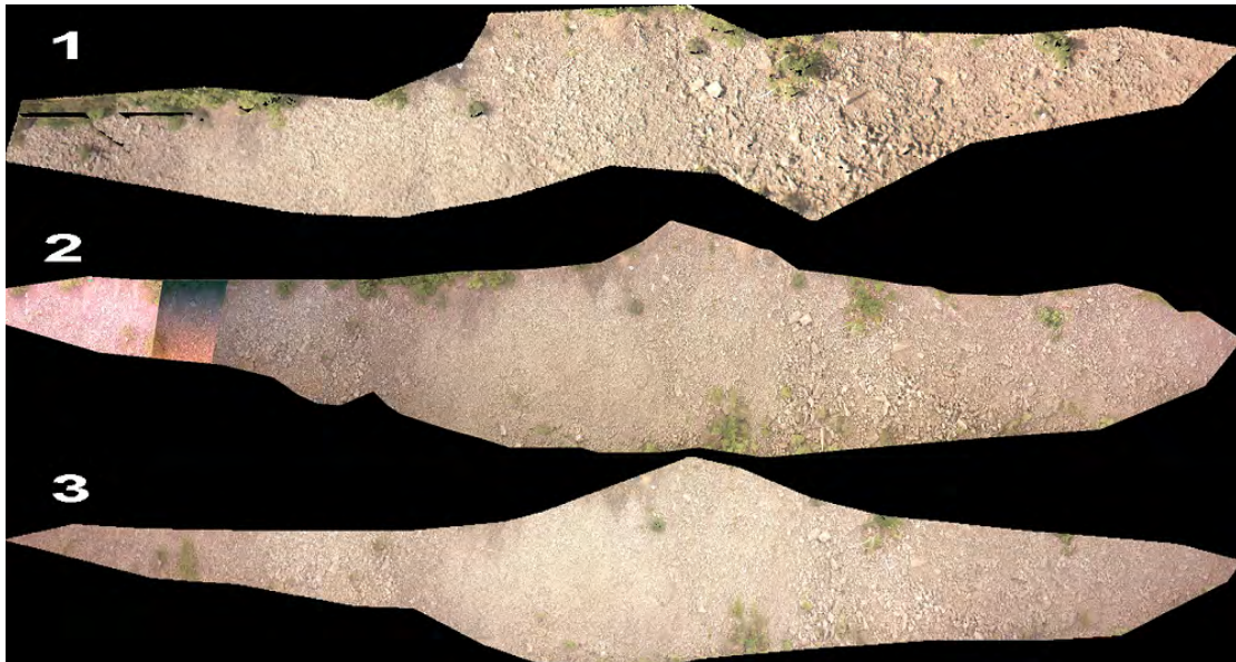
FIGURE 4.14: Image showing orthoimages from the three flights. The color anomaly seen in flight 2 appeared after Vodka processing to remove the vignette. This region was cropped out for analysis.
