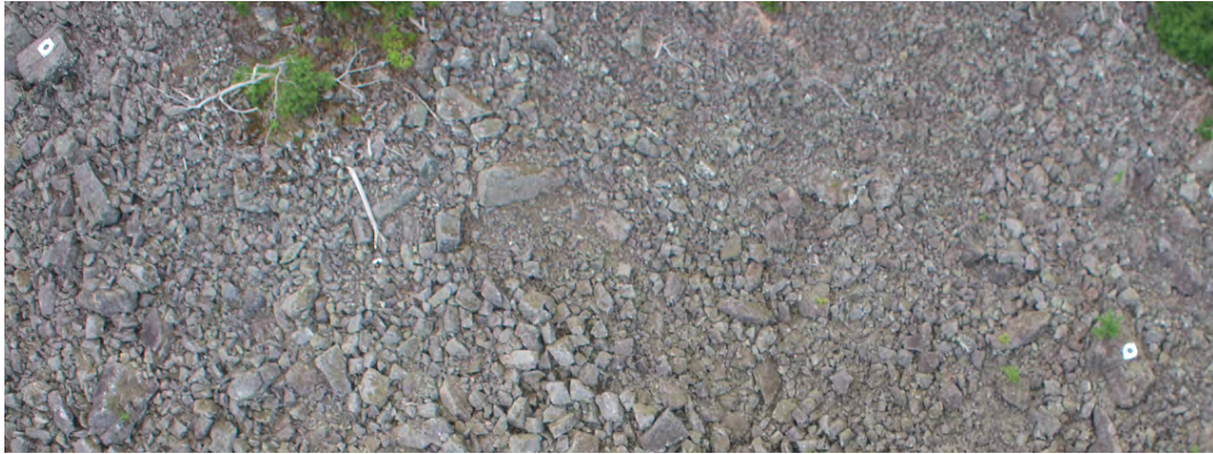
FIGURE 4.5: Photo taken from the UAV in June of 2013 of two ground control points (GCPs) survey of Kolsaas. The GCPs are 1x1m in size.
