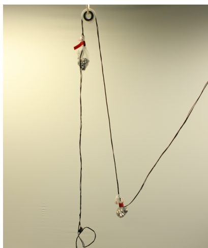
(b) An image of the pulley system used in the wiring harness.
