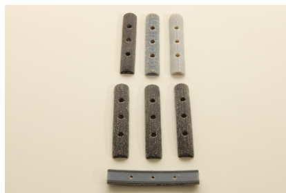
(a) An image showing multi material friction pads. Three different material mixes are used on the three topmost pads, while the back of the multi material pads can be seen in the bottom of the image.
