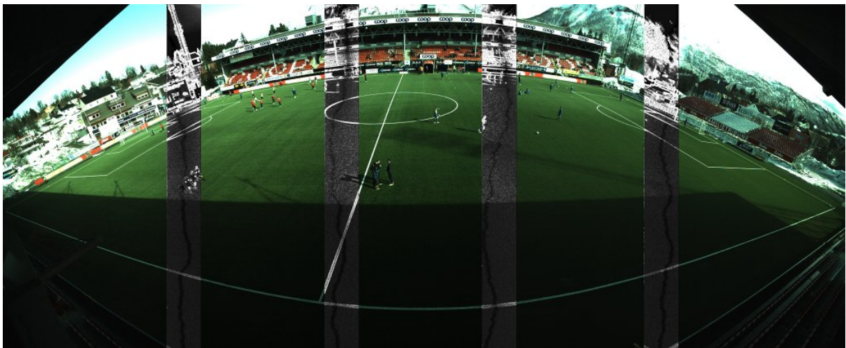
Figure 4.13: Visualization of the cost in each overlapping stitch region. White areas indicate a high cost. Note the thick transparent black “seam” in each area, the location of the previous seam that has a lower cost for nearby pixels.
