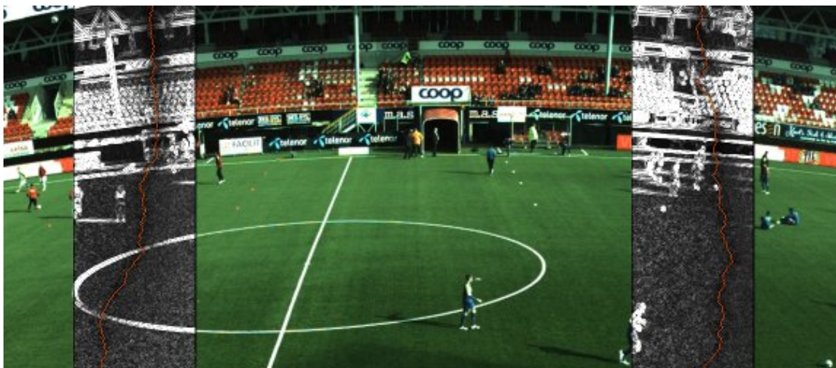
Figure 4.14: Visualization of the resulting seam, based on the cost in figure 4.13. This has been cropped to easier visualize the seam.
