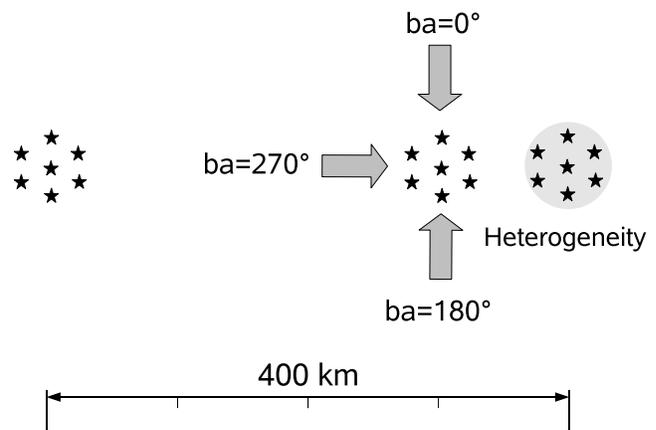
**Figure 8.** Scheme showing the locations of the arrays with respect to the location of the heterogeneity in the analysis of the variation of the phase velocity with backazimuth.
