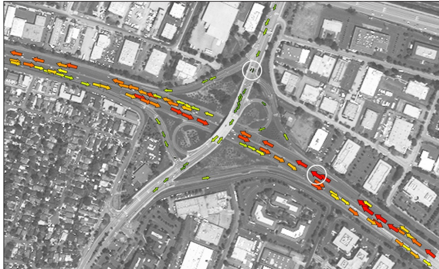
Fig. 18 Highway in Palo Alto, USA, from WorldView-2. Car velocity with colour-coded vectors according to the car speed. Dark green, upper white circle: cars waiting at traffic light ( 0 \pm 1 \text{ m s}^{-1} ). Red, right white circle: maximum car speeds of 37 \text{ m s}^{-1} ( 130 \text{ km h}^{-1} , 82 mph).
