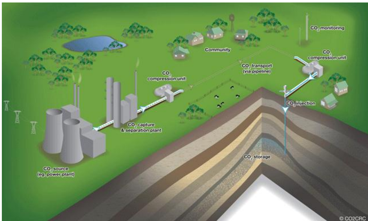
Figure 13. Illustration of the main processes at work in a CCS operation. Image source: CO 2 CRC
