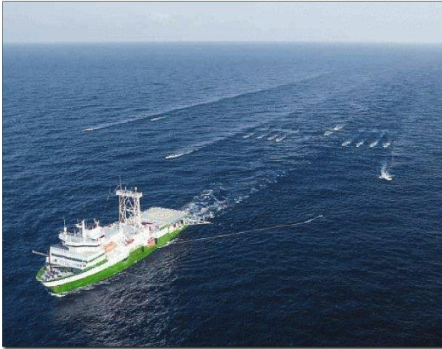
Figure 2.8: A vessel with a towed source and streamers (Picture from GeoClass, Seismic Acquisition).
