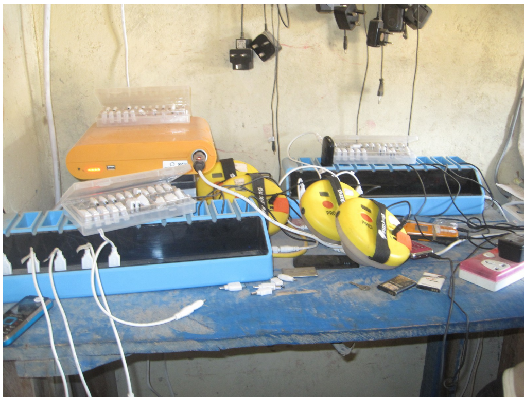
Illustration 9: The Mobisol charging system seen in use in Turkana. The system comes with a GSM modem that register the number of phones/lanterns charged. The modem is inside the “solar controller” (the yellow box). Photo: Author.
