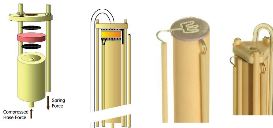
Figure 2-1: Example of connection to disk samples for impedance measurements. The schematics show principle of spring loads and regular 2-electrode 4-wire setup with dual gas supplies and thermocouple [28].
