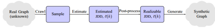
Figure 2.4 2.5K crawling and modeling approach. The original graph is first crawled to obtain a smaller sample. The values for metrics (in this case Joint Degree Distribution) are then estimated, and the sample modified accordingly to produce a generated synthetic graph. Image borrowed from [Gjoka et al., 2012]
