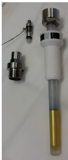
Figure 3.2: Reduction of 62 with \text{H}_2 in a sapphire NMR tube led to gold coating.
