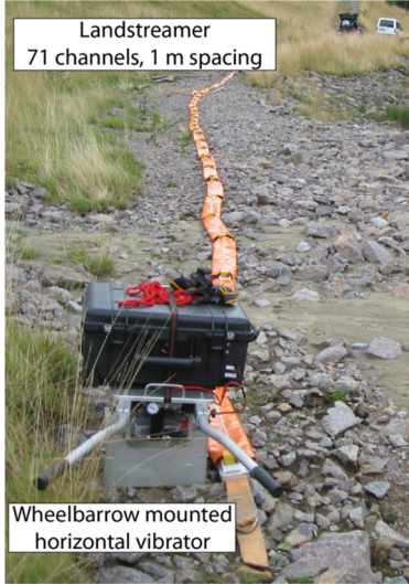
Figure 3: Pictures depicting S-wave seismic reflection acquisition using wheelbarrow mounted horizontal seismic vibrator with landstreamer along the gravel path for profile 4.
