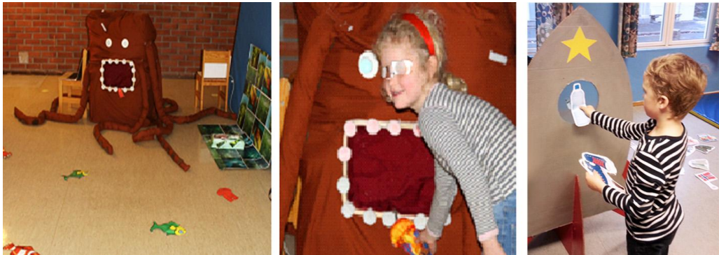
Figure 2. The re-use of technology (the mobile children's museum). On the left, octopus "Brownie" with RFID reader embedded in its mouth, middle, being fed with diverse sea creatures. On the right, same technology, but the child is packing items for the Mars mission.
