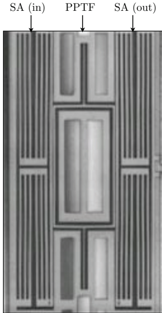
Figure 5.10: Overview of a STM 90 nm PPTF
