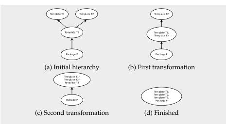
Figure 4.1: Transformation of a template hierarchy. Rewriting the instantiations is the main part of the work the JPT compiler does. This is done for arrows in this figure, from the outermost point to the innermost.
