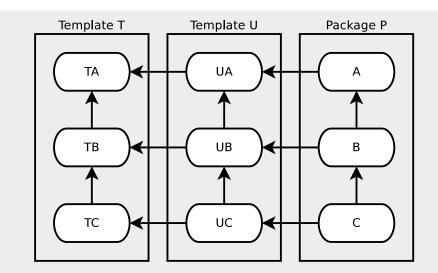
Figure 2.2: A two dimensional class hierarchy. Each class and addition class is drawn inside its template or package, with a vertical arrow pointing to its superclass, and a horizontal arrow pointing to its tsuperclass.
