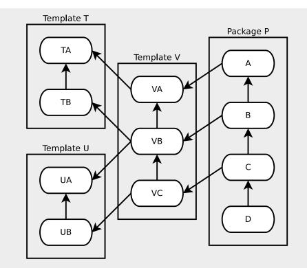
Figure 2.5: A two dimensional class hierarchy containing merged classes. Template V instantiates the templates T and U drawn in the same style as Figure 2.2. The class TB from template T and the class UA from the template U are merged to form the new class VB.
