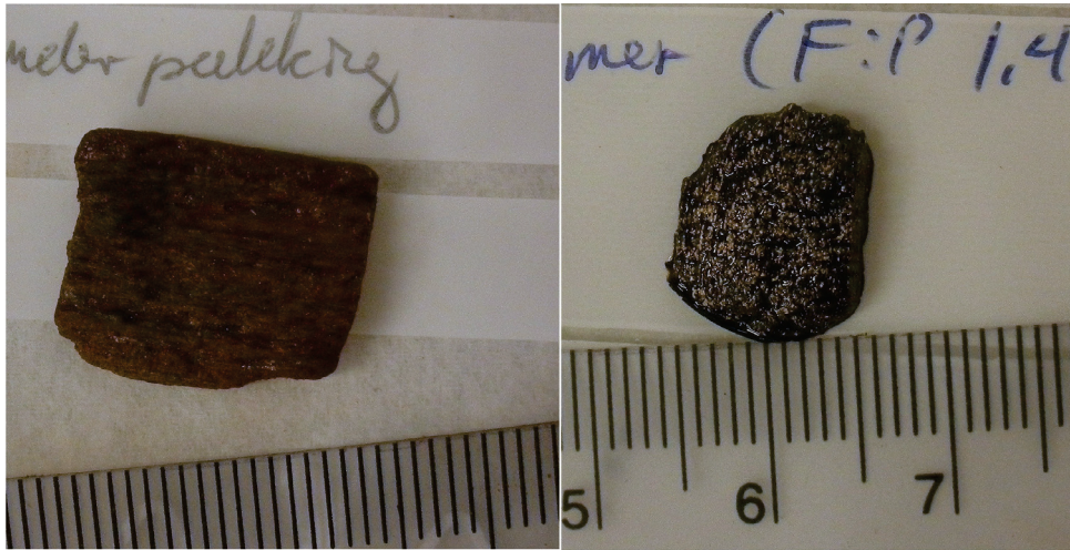
Figure 6.13: Photograph of the samples from the Oseberg find after treatment with PF. The ruler shown at the bottom of the images has a cm/mm scale. The left sample retained its wooden structure while the one to the right 'melted' during treatment. Note the shining crystals which have formed on the degraded piece to the right.
