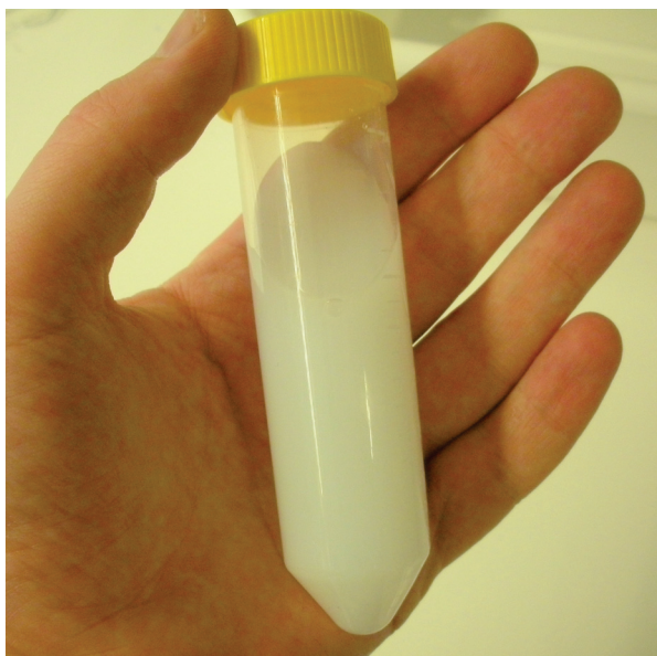
Figure 7.1: Photograph of newly collected cellulose whiskers in watery suspension.
