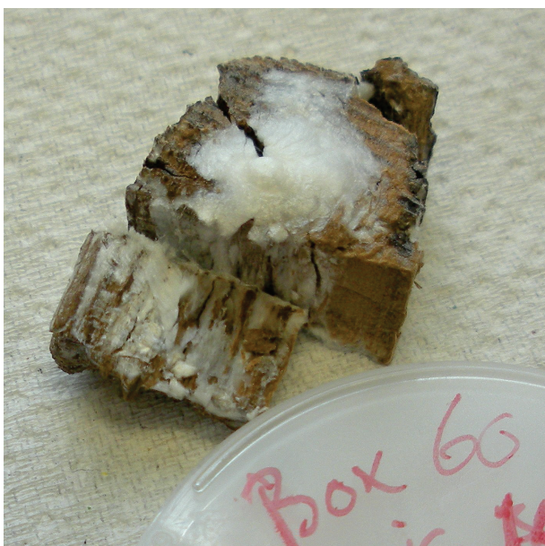
Figure 7.2: Freeze-dried piece of Viking Age wood (sample 'Box 7') impregnated with cellulose whiskers. Note how the freeze drying causes some of the whiskers out of the wooden structure. Also note that the larger cracks are filled with whiskers.
