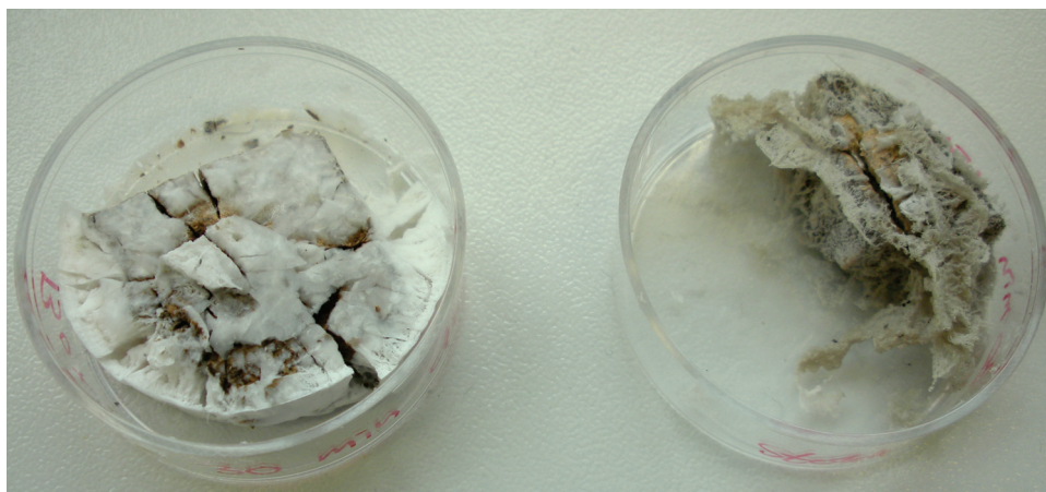
Figure 7.3: Freeze-dried Viking Age wood (sample 'Box 7') in cellulose whisker suspension. Note that the whiskers form a fluffy layer around the samples unless washed off.
