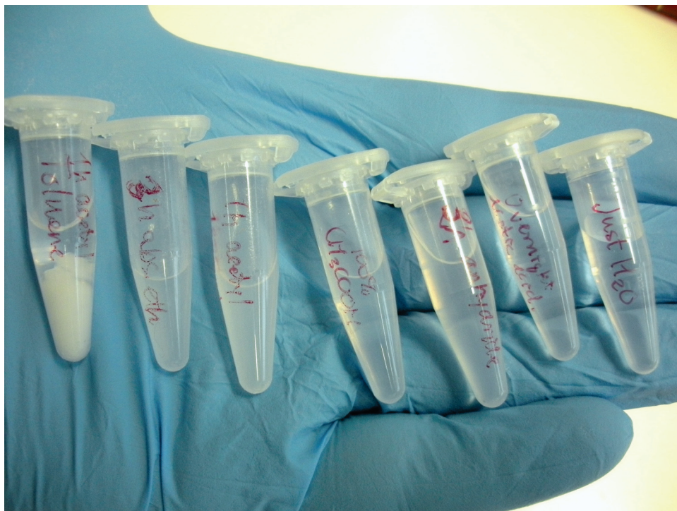
Figure 7.4: Dispersion test for a number of solvents. From left to right: Toluene, absolute ethanol, acetyl, acetic acid, acetic acid after overnight, and water: The water seemed to give the least flocculation.
