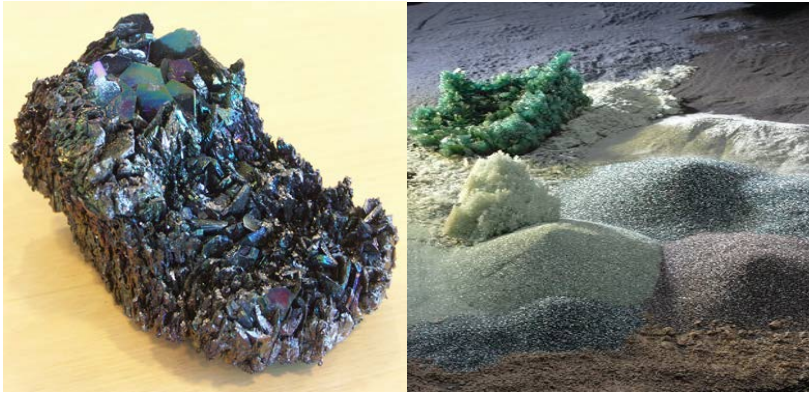
Picture group 6. Silicon carbide. To the left a silicon carbide lump from the furnace hall prior to crushing. In courtesy of Erik Bye, NIOH, Norway. To the right silico carbide lumps and final products with different grain sizes. In courtesy of Saint-Gobain Ceramic Materials.
