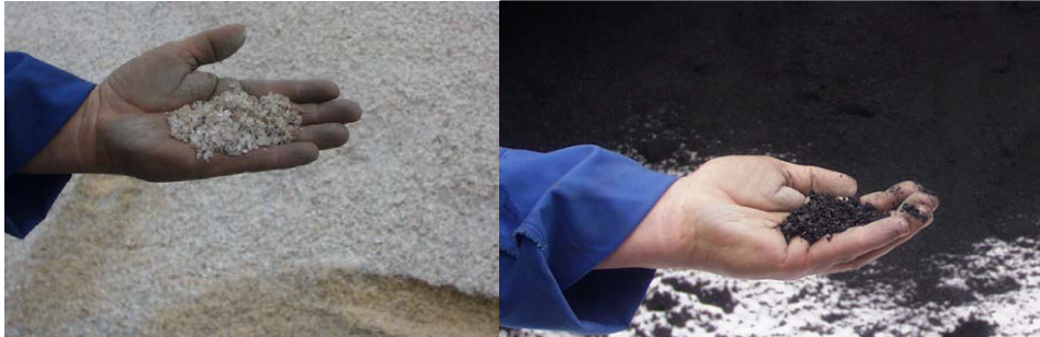
Picture group 1. The raw materials in the silicon carbide production, quartz sand (left) and petroleum coke (right).
