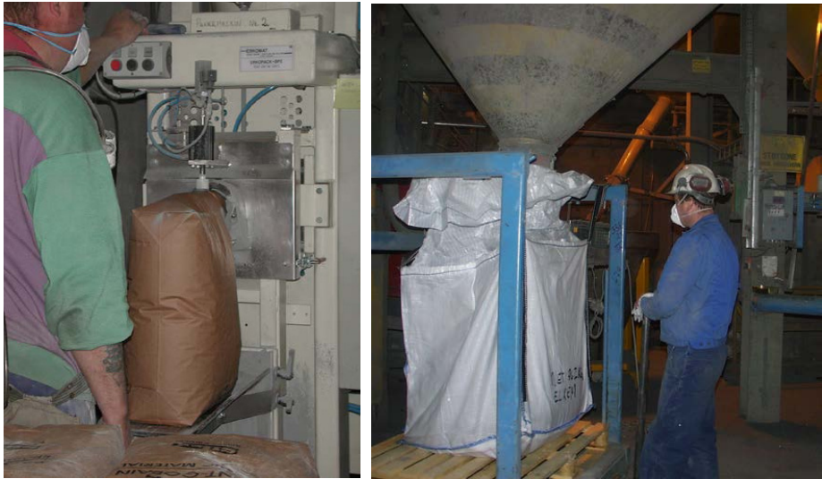
Picture group 5. Packing of SiC product in 25 kg bags (left) and big bags (right).
