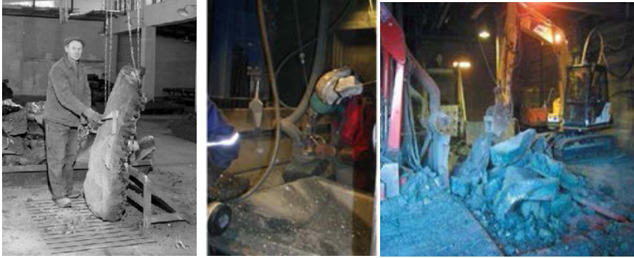
Picture group 4. Sorting the crude SiC. The picture to the left is manual sorting in 1952, the picture in the middle shows manual sorting in 2003 and the picture to the right shows sorting in cabin in 2003. In courtesy of Aust-Agder kulturhistoriske senter.
