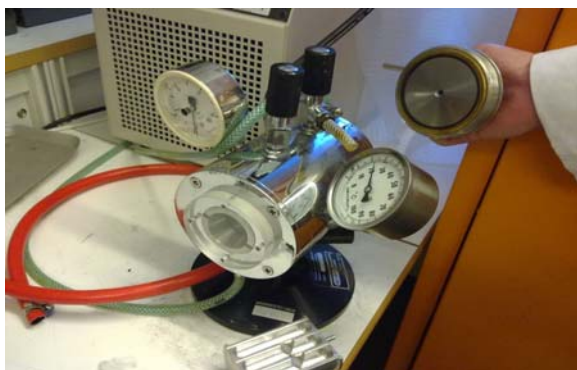
Figure 17. chamber with flowing CO 2 under high atmospheric pressure and 32°C for critical point drying.
