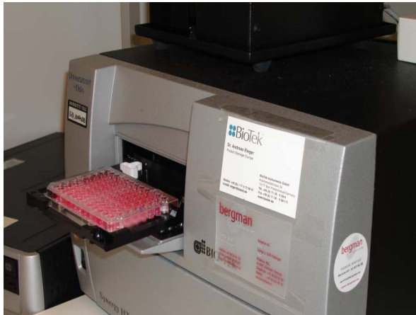
Figure 10. Spectrophotometer used to quantitate biofilms.
