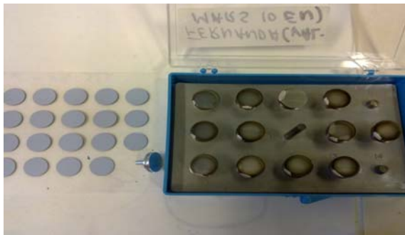
Figure 16. Discs mounted on aluminum plates to be placed in the CO 2 chamber for critical point drying.
