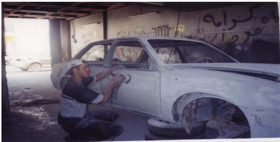
Figure 3:A worker in workshop without ventilation equipment during car painting preparation
