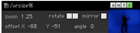
Figure 7.13: The jmod.orsize% module is used for zooming, orientating and sizing the video.
