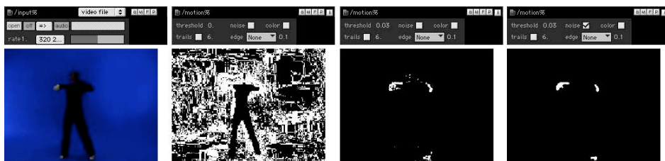
Figure 7.24: The jmod.motion% module has options for filtering and removing noise from the motion images.
