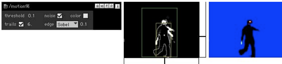
Figure 7.27: It is possible to turn on the display of running and maximum contraction boxes as well as the "centre of gravity" in the inspector panel of the module.
