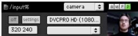
Figure 7.9: The camera pane of the jmod.input% module allows for the retrieval of live video from any video camera that works with the system, for example USB or FireWire cameras.
