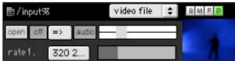
Figure 7.10: The video file pane contains controls to load and play back any QuickTime readable video file, as well as scrubbing and moving around in the video file using the timeline display.
