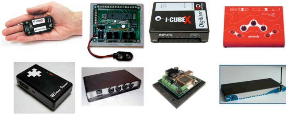
Figure 6.10: Various commercial sensor interfaces for musical or artistic purposes. From top left: the Wi-miniDig from Infusion Systems, the MIDITron by Eric Singer, the Digitizer from Infusion Systems, eo-body, WiseBox from IRCAM, Teabox from Electrotap, a Teleo module from Making Things, and a Kroonde from La Kitchen. All of these interfaces differ widely in size, number of inputs and outputs, speed, resolution, transport type, communication protocol and price.
