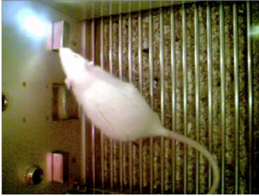
Figure 8.30: A WKY ADD rat in the experiment cage, taken from the upper right corner of the cage. The two levers that the rats are supposed to push in the experiment can be seen on the left side, each having a light above them. The feeding mechanism is seen between the two levers.
