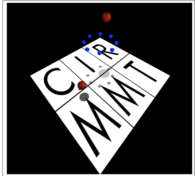
Figure 1: ViMiC Visualization: two sound sources ( red spheres ) and a virtual microphone array ( smaller, blue squares )
