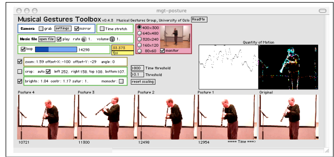
Figure 4. Example of a patch, built with the posture module, which saves a snapshot every time the change in quantity of motion is bigger than a chosen threshold value. The pictures shift from right to left, and the time code is shown for each captured frame. Here showing postures from a study of expressive gestures in clarinet performance.
