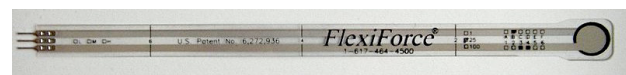
Figure 3: The Flexiforce sensor. The sensing area to the right is 9.53 mm in diameter.
