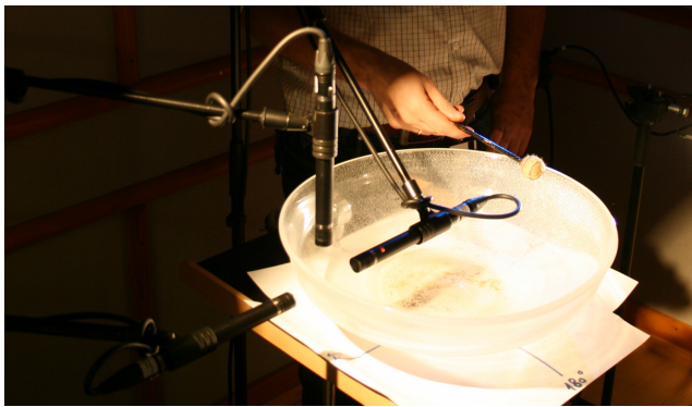
Figure 5: Microphone setup for recording sounds at the rim.
