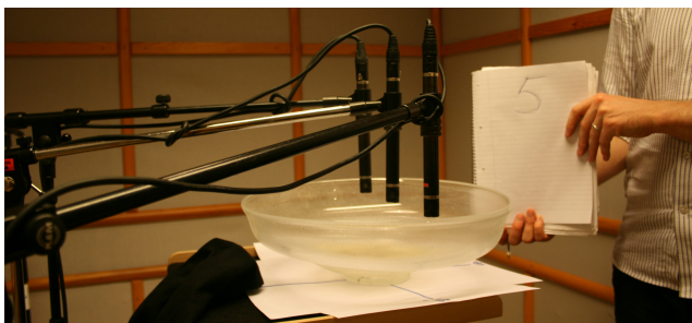
Figure 3: Microphone placement 0.5 cm above the surface, at rim, half-centre and centre positions.
