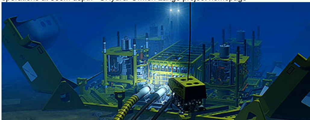
Fig 57 Artist impression of completion work on Ormen Lange sub –sea well template NOTE Protective shields folded to the sides and the exposed well-control assembly and blow out preventers. In front a Remotely Operated Vehicle (ROV) used to do the actual operations at 800m depth ©Hydro/ Ormen Lange project homepage
