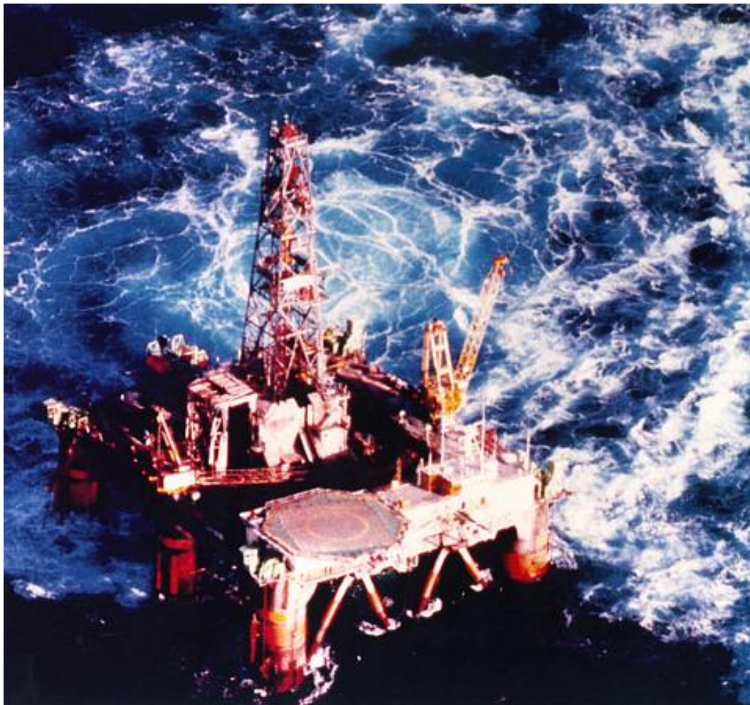
Fig 48 West Vanguard besides the gas plume from the shallow gas blowout ©Canadian Wellsite Gallery
