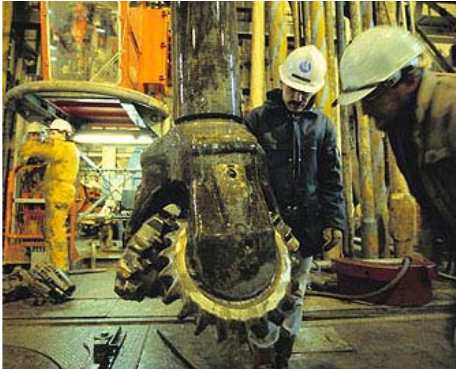
Fig 14 On the drill deck, two operators checking a large bore drill bit © Hydro
