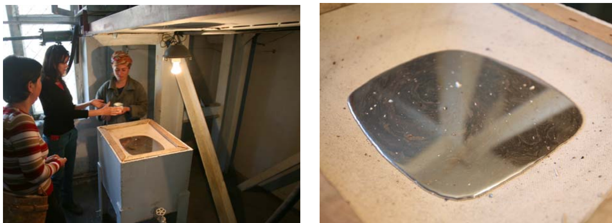
Figure 12 Filtering of metallic mercury to remove impurities after distillation
