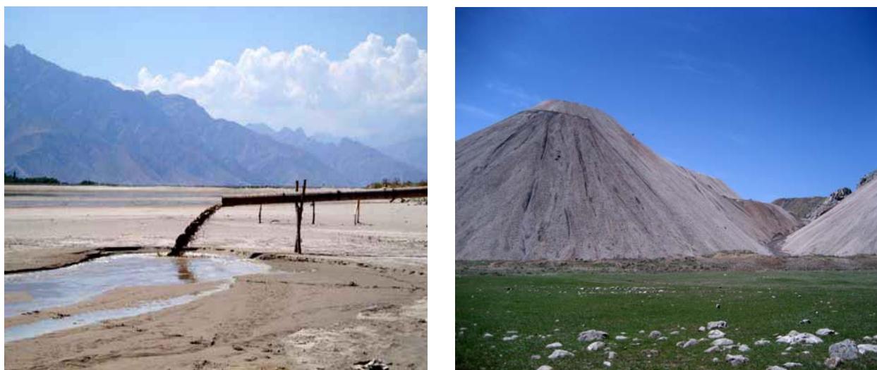
Figure 13 Tailing pond (left) and slag heaps (right) associated with KMP in Khaidarkan.
