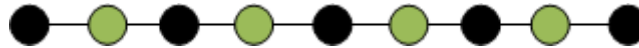
Figure 5.6: Values on the coarse, black, grid is interpolated to the fine grid, green, using linear interpolation.
