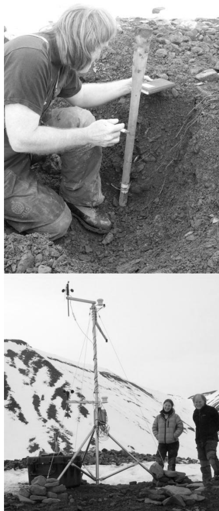
Figure 21: Installing debris layer thermistors (above). After final adjustments of weather station (below) (Photos by J. Mertes).
