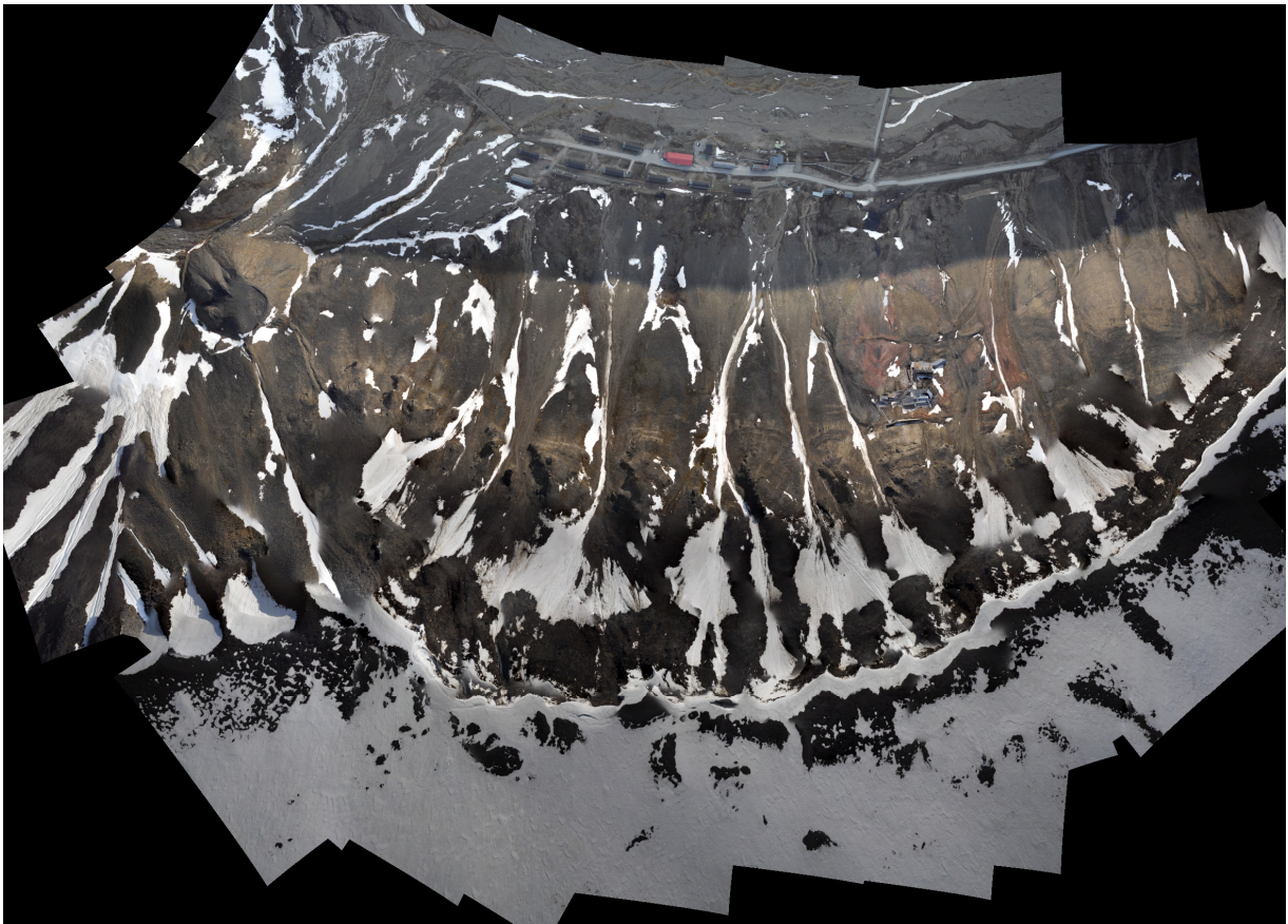
Figure 27 Aerial mosaic of 112 images taken 680 m above the valley bottom on 20 June 2010. The Gruvefjellet plateau and ridgeline are in the lowermost part and the houses of Nybyen in the upper part of the picture. The snow cover in the Gruvefjellet slope section is uncontinuous and talus cones are visible at the terminus of the five gullies. © KOLIBRI GEO SERVICES
