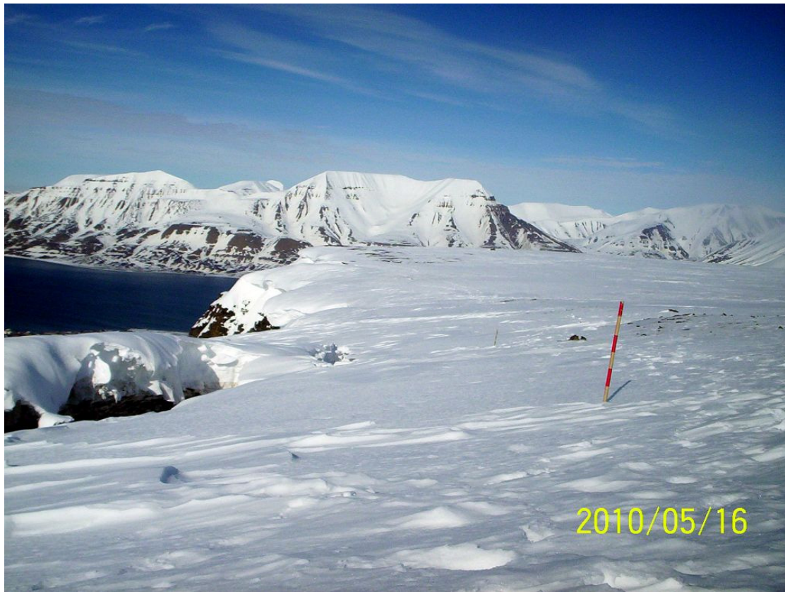
Figure 17 Automatic time lapse photograph of the 'Gruvefjellet' camera from 16 May 2010. The coloured height indicators on the snow depth measuring stake represent 10 cm. Note the opening cornice crack in the foreground on the left side
