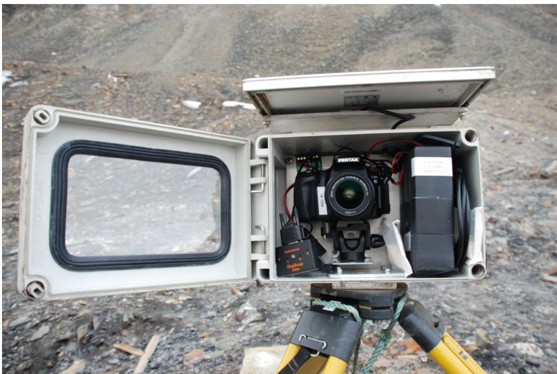
Figure 13 The automatic time lapse camera set-up of 'Sverdrupbyen' installed in a weather proof box and mounted on a tripod. The time lapse controller is to the left of the digital camera and the 12V battery to the right. The solar panel is fixed on the weather proof box.
