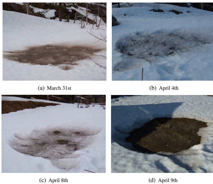
Figure 2.1: (a), (b), (c), and (d): Ash was applied to the snow pack in Hjartdal early in the melt season. The snow depth was 53 cm when the ash was distributed evenly over the snow on March 31st 2009. The contaminated area was completely melted within 9 days , while the surrounding snow pack melted in 13 days . A second patch of ash that was more exposed to sunshine also hastened the snow melt by 4 days , from 9 to 5 days in total. Photos by Bjørg Aamaas and Thorbjørn Aamaas.
