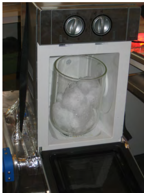
(b) A snow sample ready for melting
