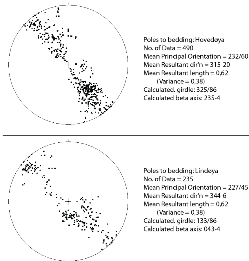
Fig. 4.1 Stereographic projections displaying all bedding planes measured in the field of the two islands ( Hovedøya, n=490 and Lindøya, n=235) within the study area.
