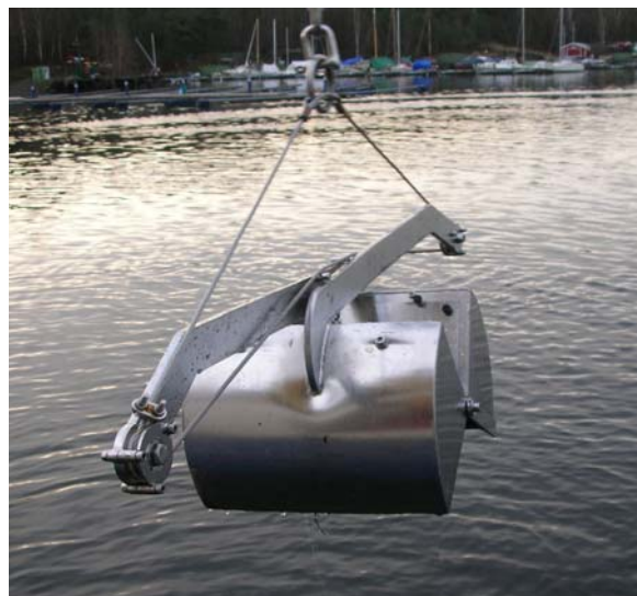
Figure 3.2 Equipment for sediment sampling
