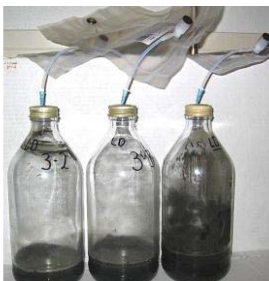
Three gas test jars with gas bags inserted into the rubber membranes
