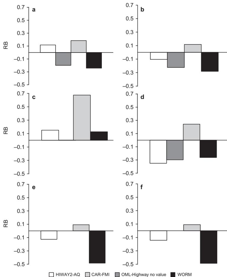
**Fig. 4.** Relative bias (RB) for all models applied to the Norwegian (station 3), Danish (station 2) and Finnish (VAN station) data. (a) Norwegian (station 3) non-normalised, (b) Norwegian (station 3) Q-normalised, (c) Danish (station 2) non-normalised, (d) Danish (station 2) Q-normalised, (e) Finnish (VAN station) non-normalised, (f) Finnish (VAN station) Q-normalised.
