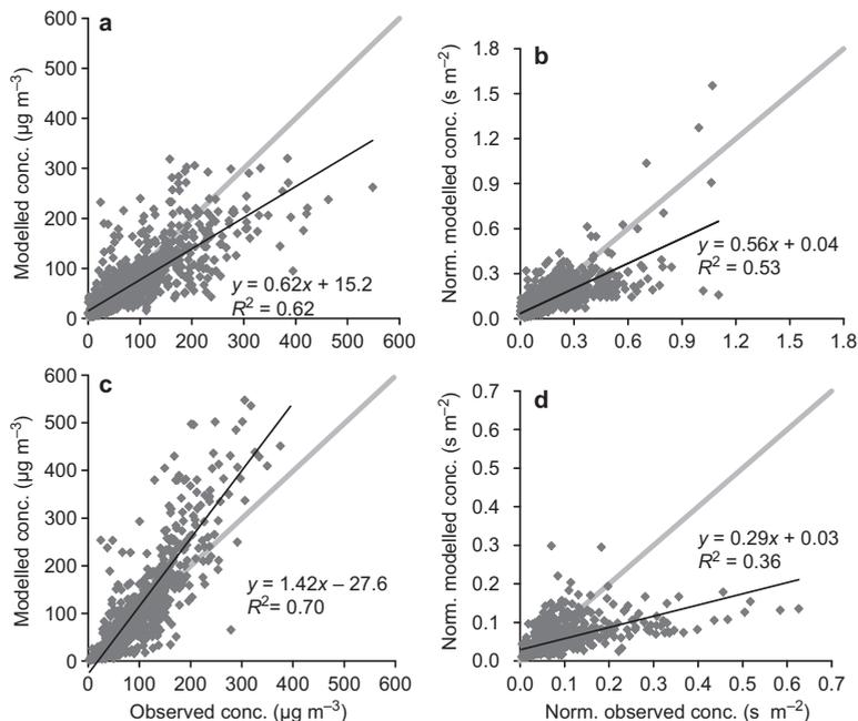
**Fig. 3.** Scatter plots of modelled versus observed concentrations, for (a) OML: Norwegian data (station 3) non-normalised, (b) OML: Norwegian data (station 3)  $Q$ -normalised, (c) WORM: Danish data (station 2) non-normalised, (d) WORM: Danish data (station 2)  $Q$ -normalised. Included in the plots are the one-to-one line (grey line) and the linear regression fit (black line), with the regression model and coefficient of determination ( $R^2$ ).
