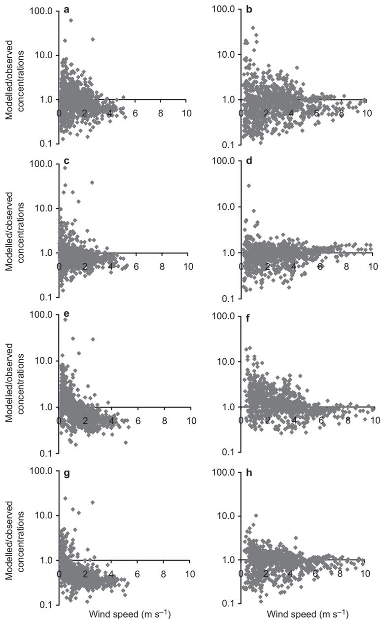
**Fig. 5.** Scatter plots of the ratio of modelled to observed concentrations *versus* wind speed at 2 m above ground for all models applied to the Norwegian (a, c, e, g: station 3) and Danish (b, d, f, h: station 2) data.
