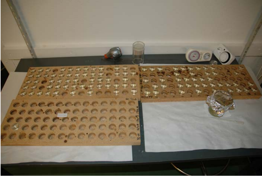
Fig. 5 Cardboard tables with 5x14, 12.5 mL beakers, extra table (left bottom) for handling of juveniles.
