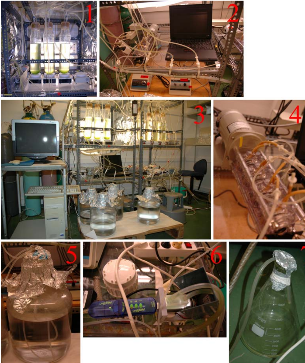
Fig. 4 Chemostat set-up: 1. Sealed flasks with algae, 2. Laptop computer connected to Lux-meter, peristaltic pumps (left), power supply and controllers to peristaltic pumps (bottom), 3. Overview, computer (left) controls the on/off cycles through a relé (not depicted) of the peristaltic pumps, 4. One of the two sets of peristaltic pumps, 5. COMBO-water with inlet tubes to the chemostat, 6. Lux-meter (left), cuvette (middle, with tubes) and LED light (inside box, right), 7. Outlet-water from the chemostat.
