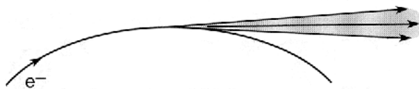
Figure 3.7 Radiation occurring when a relativistic electron travels in a uniform magnetic field, executing a circular motion with acceleration directed toward the centre. Figure taken from Atwood (83).
