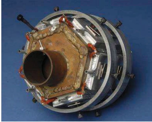
Figure 2.6: A ten-year old exhaust thermoelectric prototype from General Motors. Picture from General Motors, USA.
