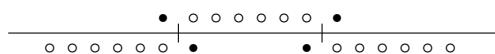
Figure 4.7: A one dimensional grid, with sub grid computational points ( \circ ) and ghost points ( \bullet ).
