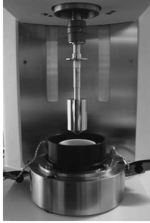
Figure 4.6: The rheometer used for electro and magnetorheological measurements.
