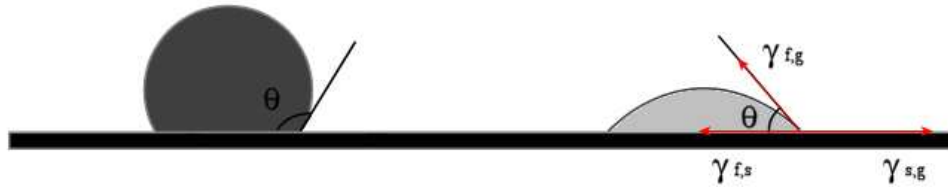
Figure 2.5: a) A non-wetting droplet placed on a plane solid surface. The solid and fluid are surrounded by wetting gas. The contact angle \theta > 90^\circ . b) Same as in a) , but the droplet of fluid now wets the solid. Also included are the surface tension vectors between the different phases, drawn from one of the contact points. \theta < 90^\circ
