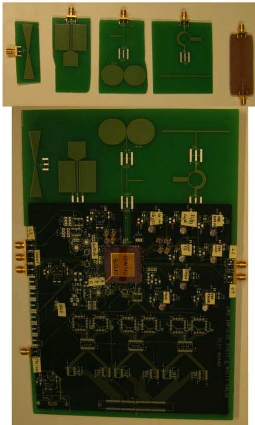
Figure E.2: Shows the PCB with minimum connection points and antenna structures used during measurement. Top left is the pulse shaping strip-line tested for generating dual sloped monocycles.
