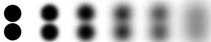
Figure 2.7: Two point sources side by side with added blur until the objects can no longer be separated
