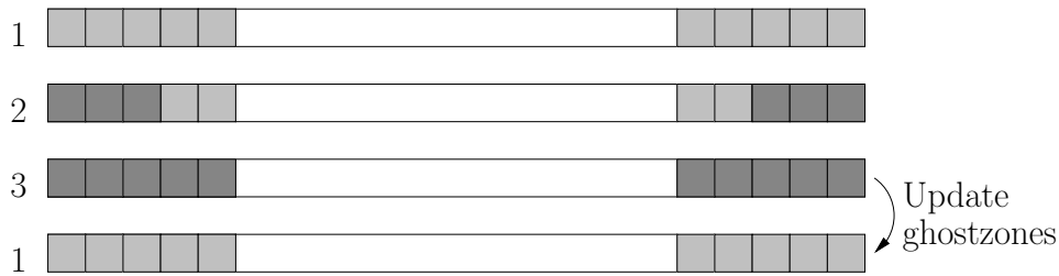
Figure 6.4: Ghostzones that can be trusted after the different steps in the algorithm. Ghostzone with reliable values (light grey), ghostzone with unreliable values (dark grey) and subdomain (white). 1: Before prediction. 2: After prediction. 3: After correction.
