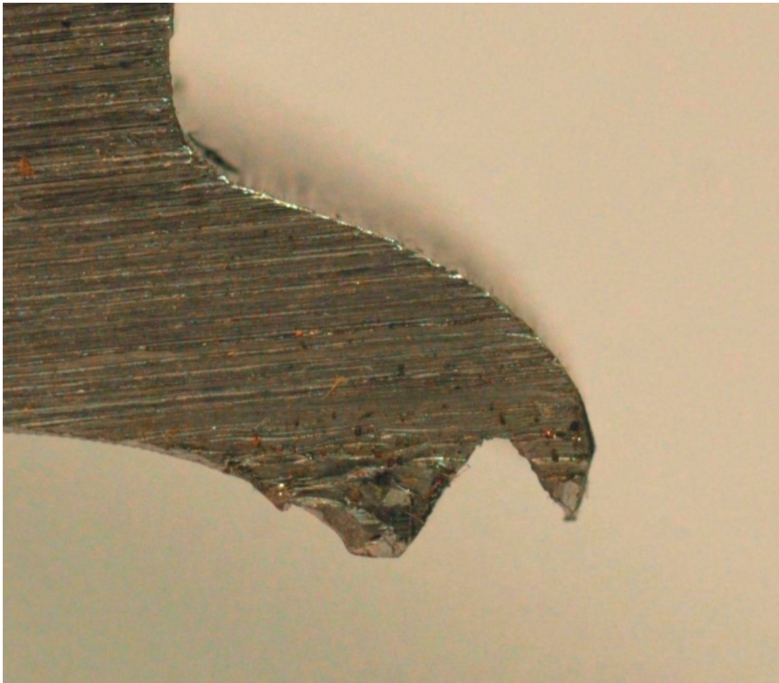
Figure 7.27: Macro photography of notch section
