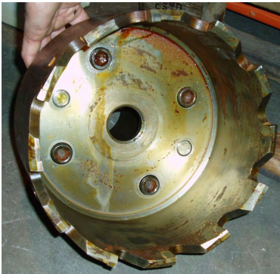
Figure 2.16: The core drill saw [6]
