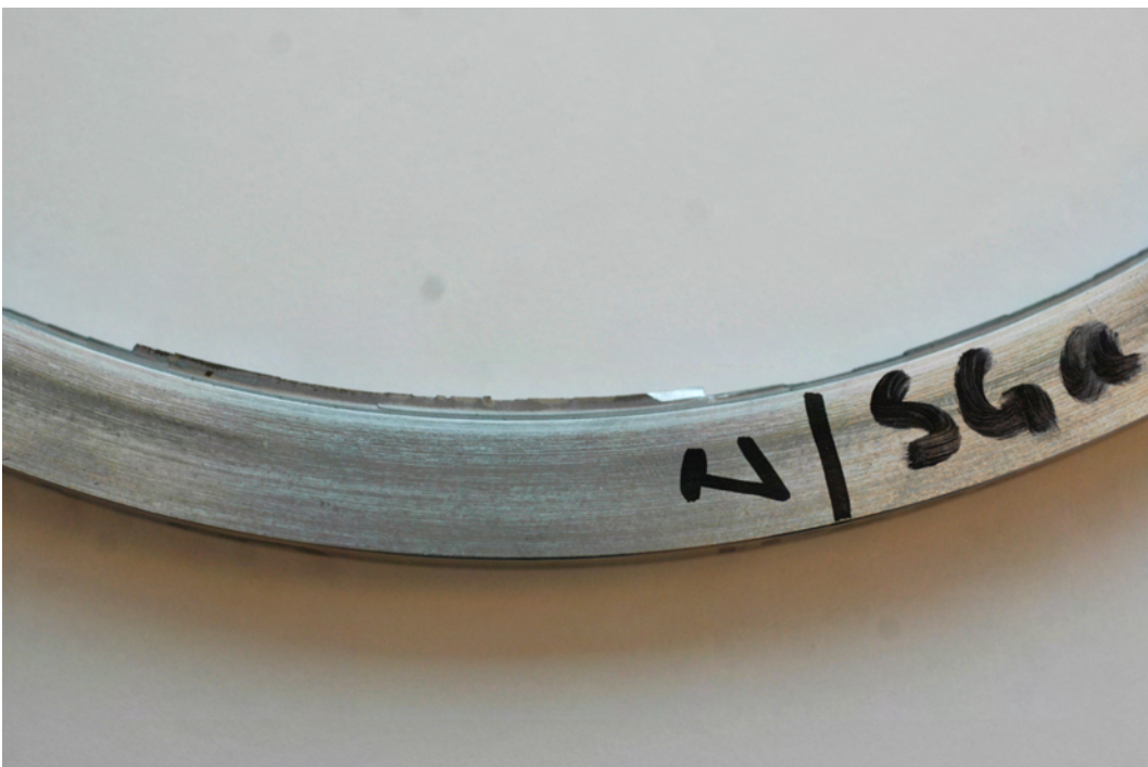
Figure 7.29: Photo of fracture initiation zone, membrane support ring
