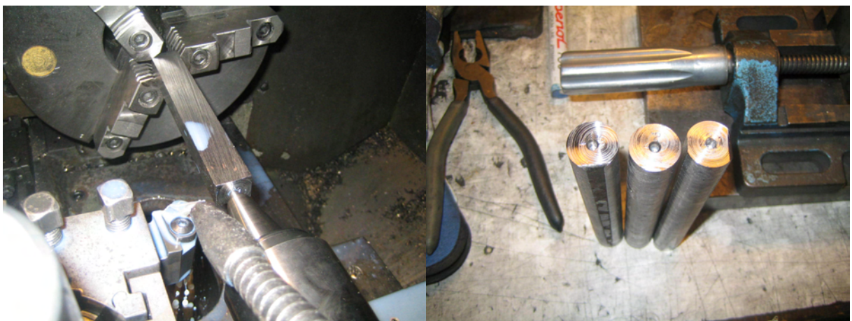
Figure 4.10: Machining of test specimen
