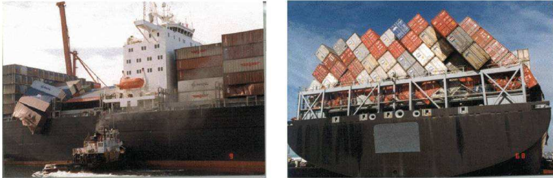
Figure 1.2: APL CHINA container damage.
