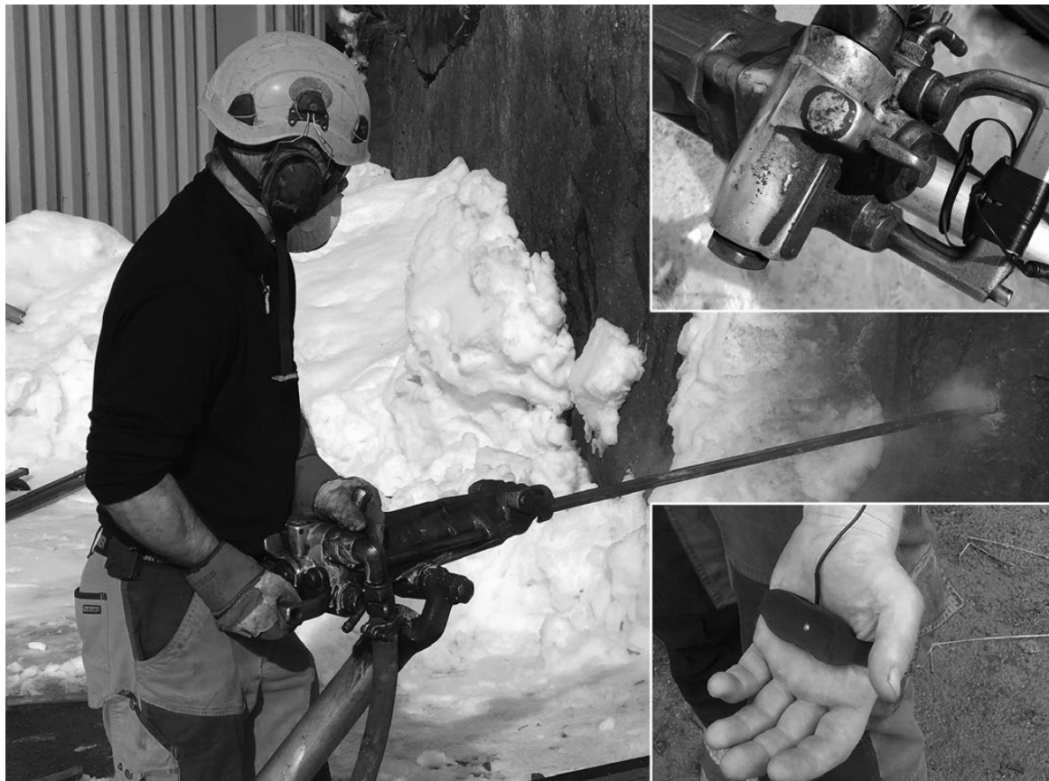
Figure 1. Work process (jackleg drilling) done for simultaneous measurements with tool-attached (upper right in picture) and hand-attached (lower right) accelerometers.
