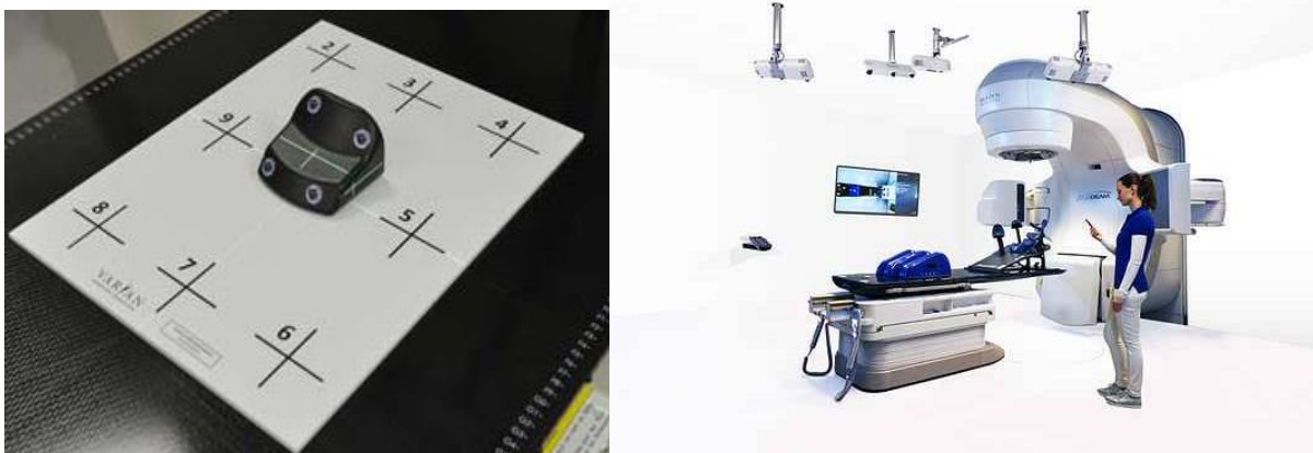
Figure 2.26: Illustration of the Real-time Tracking and Motion Management system from Varian on the right and picture of the marker block on the left [51]
